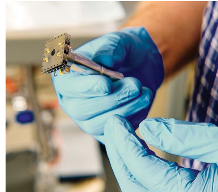
Donovan is holding a diagnostic that will be installed in the UT Plasma Exposure Stage to measure the ion temperature.
